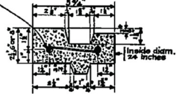
CROSS SECTION OF REINFORCED CONCRETE RING
