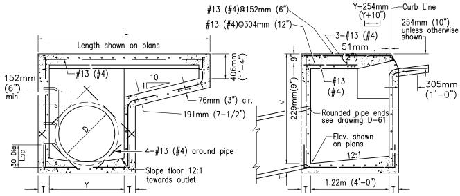
Determined by pipe size-1.22m (4') min., 2.44m (8')max.
