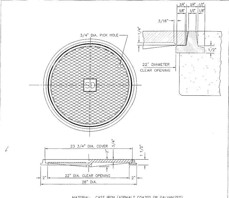
MATERIAL: CAST IRON (ASPHALT COATED OR GALVANIZED)
