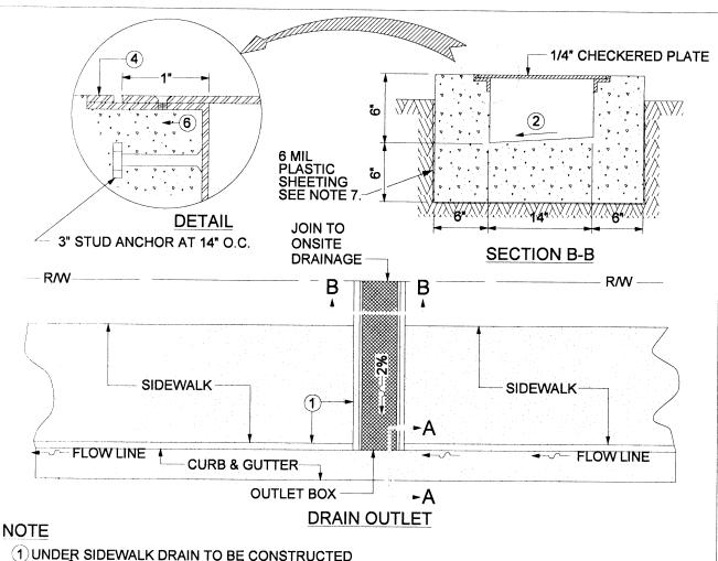
1 UNDER SIDEWALK DRAIN TO BE CONSTRUCTED AT 90%. VARIATIONS FROM 90 REQUIRE THE APPROVAL OF THE DIRECTOR OF TRANSPORTATION.
